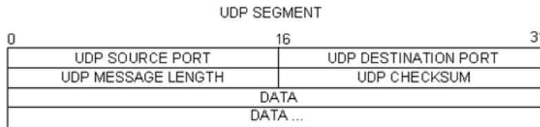
Using the Wireshark capture of the first UDP datagram, fill in information about the UDP header. The checksum value is a hexadecimal (base 16) value, denoted by the preceding 0x code:
