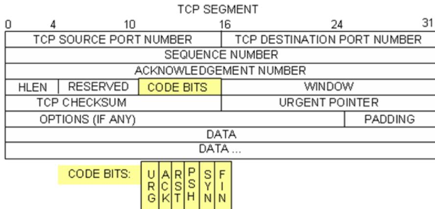
The image above is a TCP datagram diagram. An explanation of each field is provided for reference:
